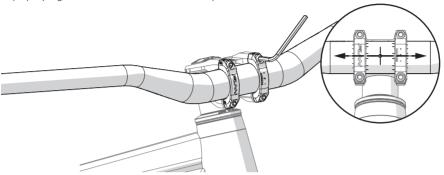
Once the new bar is in place, adjust its roll angle, which affects wrist comfort and bike control. Then, tighten the stem's faceplate in a cross pattern for even pressure distribution.
