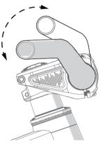
5. Reattach the components you previously removed onto the new handlebar, ensuring they are positioned for optimal comfort and accessibility.
