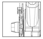
**Step 1:** Install the mounting plate (without the top guide) directly onto the tabs.
